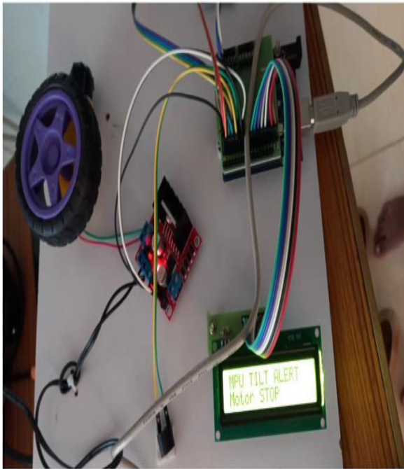
Fig 7: Vehicle Tilt Detection and Safety Control Using MPU Sensor
